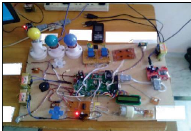
Fig: 3 Industrial Home Monitoring using Atmega 328
